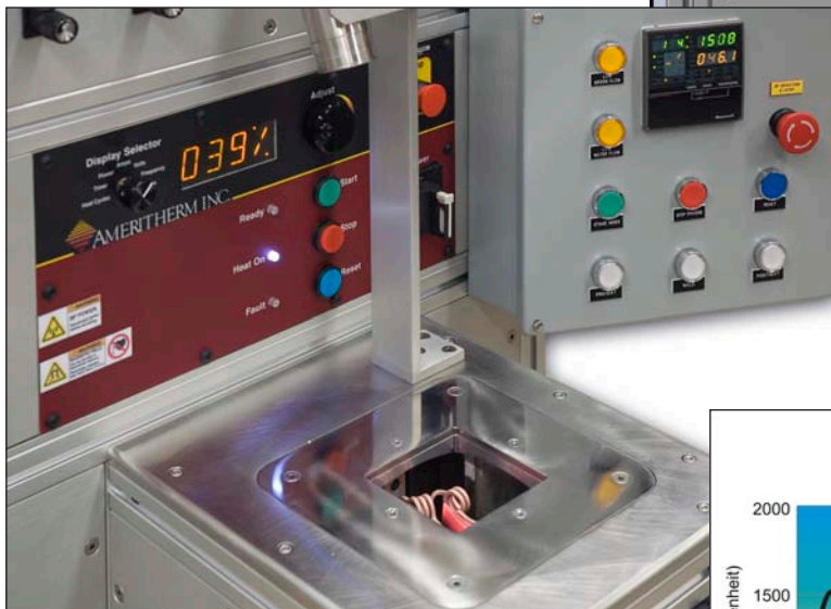
Power supply, control panel and work area
