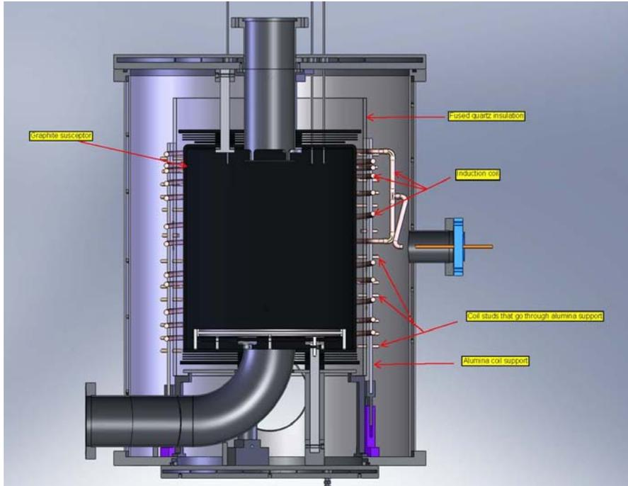
Cross section of an Induction High Vacuum Furnace
