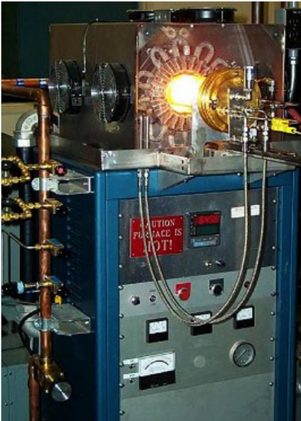
High vacuum, infrared system at ORNL
