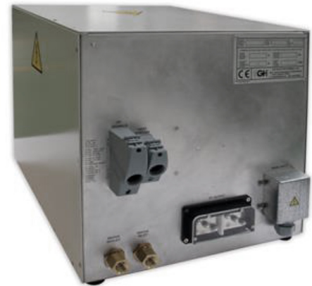
20 kW rear panel layout - 1/2" NPT water connectors; bushing type for main input and HF output
